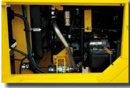
EASY ENGINE ACCESS Engine cover doors on right and left sides provide easy access for maintenance.
